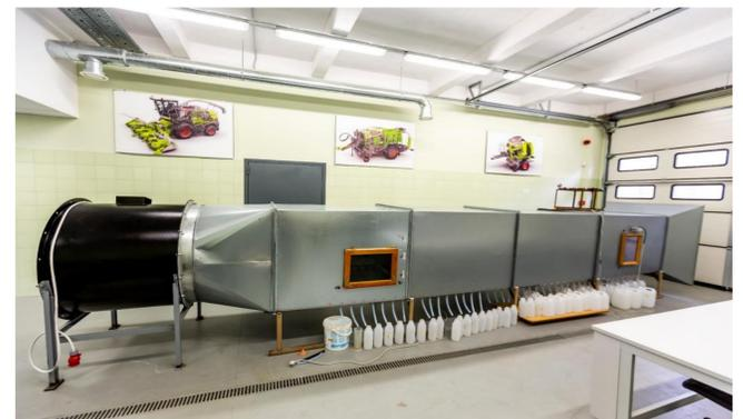
Fig. 1. Test bench (wind tunnel) for spray drift investigation (Bauša et al., 2017): 1, frame; 2, suction fan with electric motor; 3, 13, air flow straighteners; 4, 11, window; 5, air velocity measurement place; 6, flask; 7, connection chamber; 8, investigation chamber; 9, spray supply equipment; 10, nozzle; 12, corrugated tin; 14, air intake section
