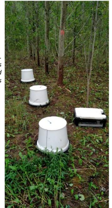
Fig. 2. Measurements with closed chambers
